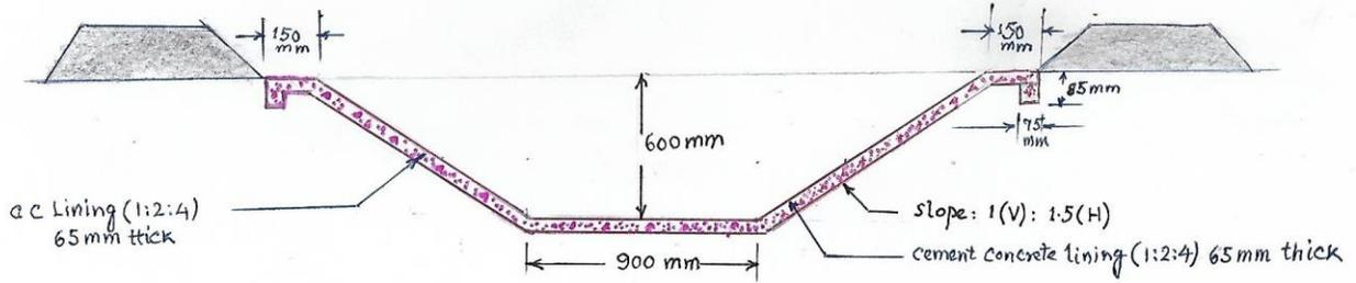
NOTE: LENGTH OF MODEL SECTION along FLOW = 600 mm
